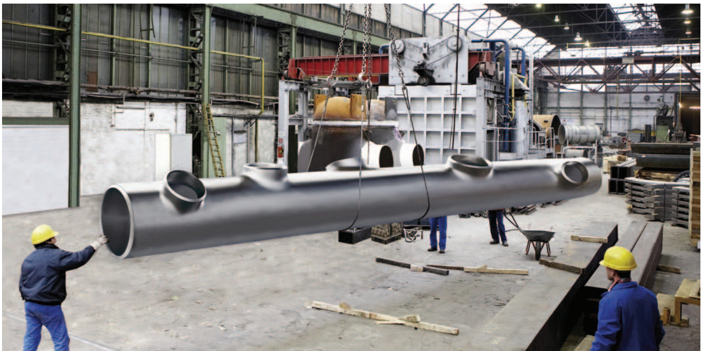
With the new, hot forming press Schulz is able to produce seamless extruded headers and tees up to 48" in size.
